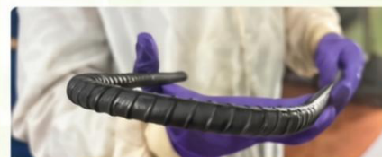
No cracking at outside radius of the bent bar
