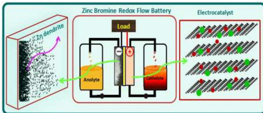
Fig. 2 Metal halides ( $\text{ZnBr}_2$ ) redox flow battery
