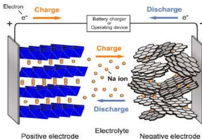
**Figure 2 The working principle of a typical sodium-ion battery Adopted from: Chemical Reviews 114 (2014) 11636**
