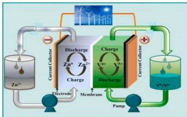
Fig. 3 Metal-Metal hybrid redox flow battery
