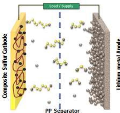
Figure 1 Architecture of a typical Lithium Sulfur Cell
